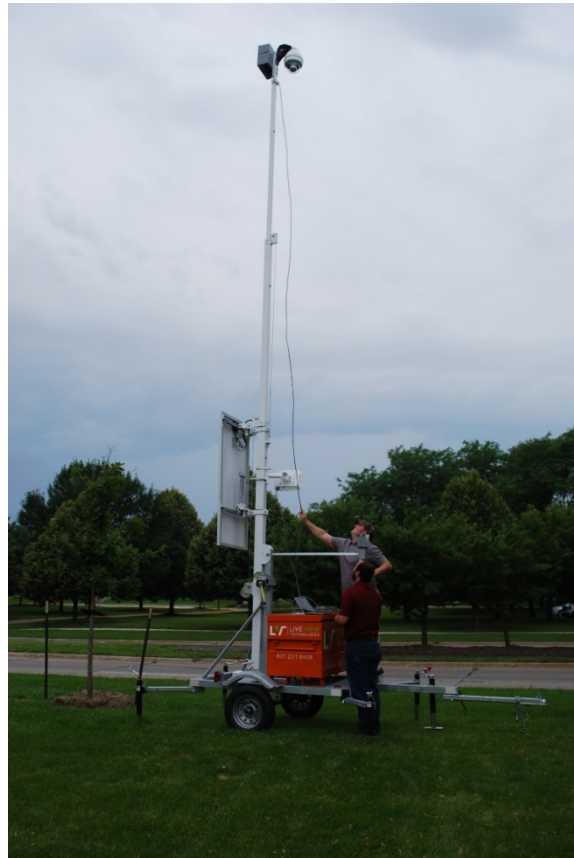
Figure 8: Video Data Collection Array
